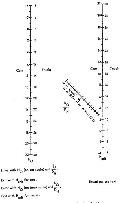
Barrier Nomogram B3. Calculation of the Quantity H<sub>crit</sub>.
