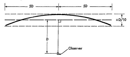
Figure A-1. Permissible Curvature for Approximately Straight Roads.
