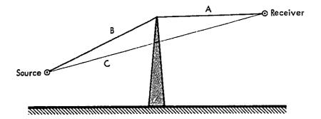
Figure B-2. Illustration of Path Length Difference ( $\delta = A + B - C$ ).
